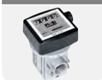
Flow rate: 20 -220 l/min Accuracy: +/- 1% Oval gear system Code: FO0540000
